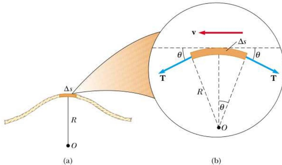
**Figure 16.11** (a) To obtain the speed  $v$  of a wave on a stretched string, it is convenient to describe the motion of a small element of the string in a moving frame of reference. (b) In the moving frame of reference, the small element of length  $\Delta s$  moves to the left with speed  $v$ . The net force on the element is in the radial direction because the horizontal components of the tension force cancel.
